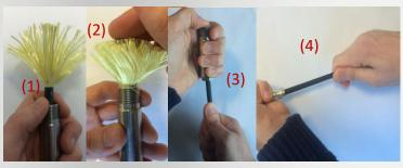
In vertical position, fibers are positioned around the termination (in a uniform way) (1). Place the spike in the center of fibers (2) then pull downwards the cable to put back the spike in the cable (3). Once connected, pulled repeatedly to exercise a first tension to the cable (4).
