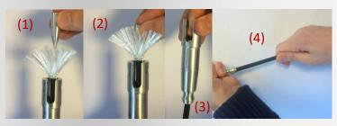
In vertical position, fibers are positioned around the termination (in a uniform way) (1). Place the spike in the center of fibers (2) then pull downwards the cable to put back the spike in the cable (3). Once connected, pulled repeatedly to exercise a first tension to the cable (4).
