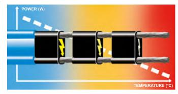
**NB**: unlike the other heating elements, it is impossible to check that a self-regulating cable is operating correctly by measuring resistance with an ohmmeter. This can be done instead by measuring the voltage/current.
